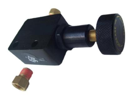
**Installation** – The proportining valve is intended to be installed in the rear fluid line after any factory style distribution block. An adjustable proportining valve should never be installed between the master cylider and distribution block as the block will sence unequal pressure and block fluid flow.
