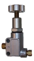
**Installation** – The proportining valve is intended to be installed in the rear fluid line after any factory style distribution block. An adjustable proportining valve should never be installed between the master cylider and distribution block as the block will sence unequal pressure and block fluid flow.
