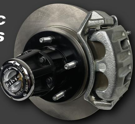
Features direct fit to factory knuckle, 51mm 2 piston zinc plated caliper, 12" vented brake rotor, grade 8 mounting hardware, precision CNC-machined mounting brackets. Works with stock and aftermarket lockout hubs.
